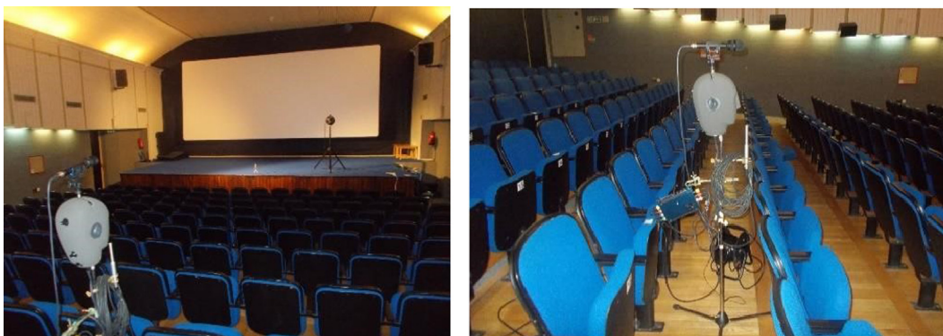
Fig. 5. Sound source and microphones during the acoustic measurements.
