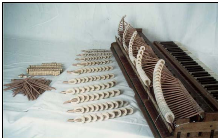
Fig. 2 - Replica of hammer-set in the Rossini's Pleyel
